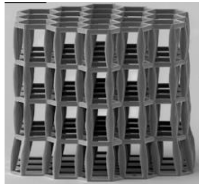
Hexagonal structure coated with \text{Al}_2\text{O}_3 (ALD) for multiscale materials towards lightweight applications
